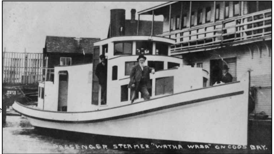
The pristine 65-foot Wah-ta-waso (aka Watha Wasa) shortly after her construction in 1910. Moved by a steam engine-driven propeller, the boat was reliable, fast, and not dependent on wind and tide.
